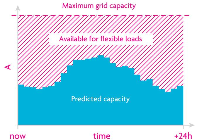
Figure 7: Maximum grid capacity vs. predicted capacity and flexible loads
