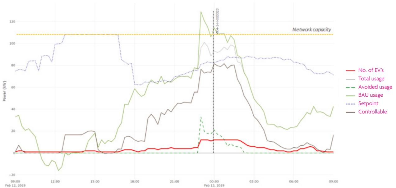
Figure 11: Visualization of load profiles for dynamic charge management
