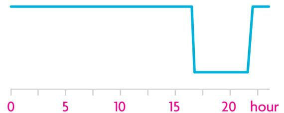
Figure 4: Example daily static control signal for EV charging
