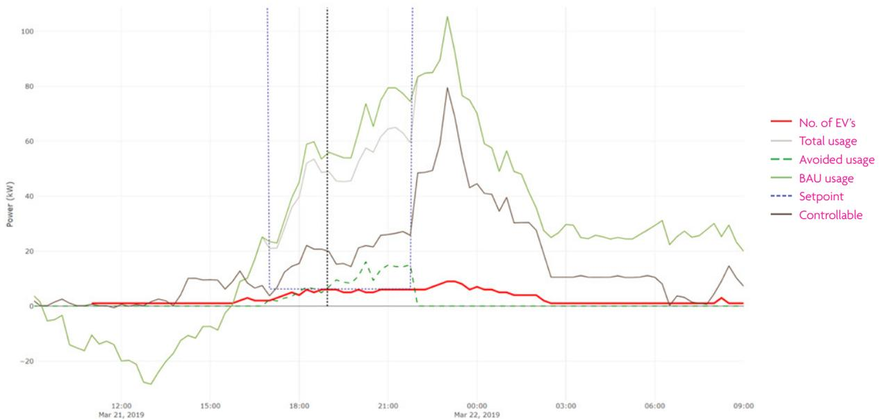
Figure 12: Visualization of load profiles for static charge management
