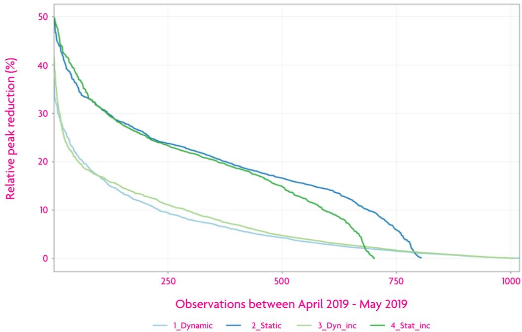
Figure 21: Duration curves of relative peak load reduction with maximum constraint
