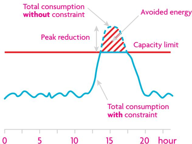
Figure 5: Determining how charge management reduces peak load
