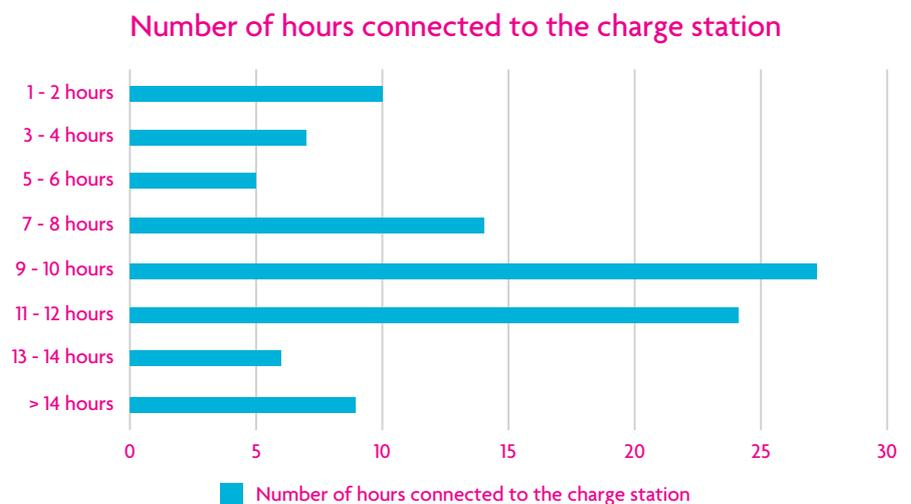
Figure 16: Average number of hours that the EV is connected to the charge station
