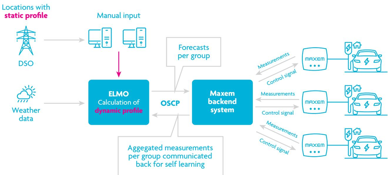
Figure 6: Overall technical architecture
