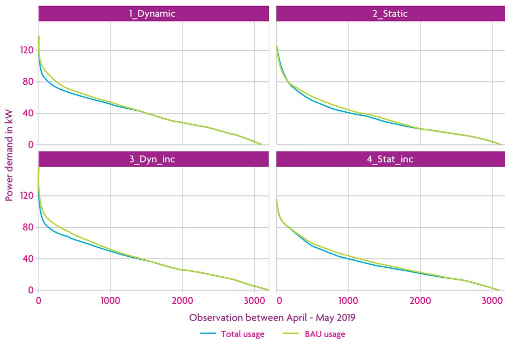
Figure 22: Duration curves of total usage and BAU usage with maximum constraint
