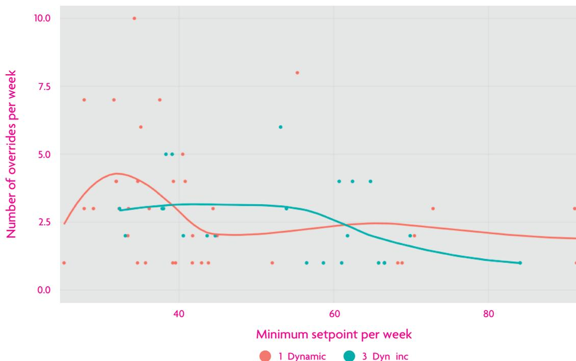
Figure 23: Correlation between the number of overrides and setpoint for the dynamic signal groups
