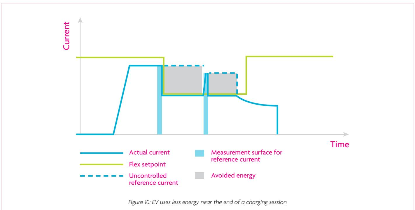
Since the avoided energy cannot be *measured*, the method described above was developed to *calculate* it. Because the firmware was adapted to handle these three scenarios, researchers can make an accurate calculation about the actual impact of charge management.
