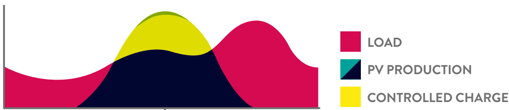
Charge control: Electric vehicle only charges when a surplus of solar power is available.
