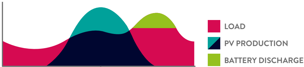
Peak Shaving: Solar production is stored to later reduce the peak load on the grid.
