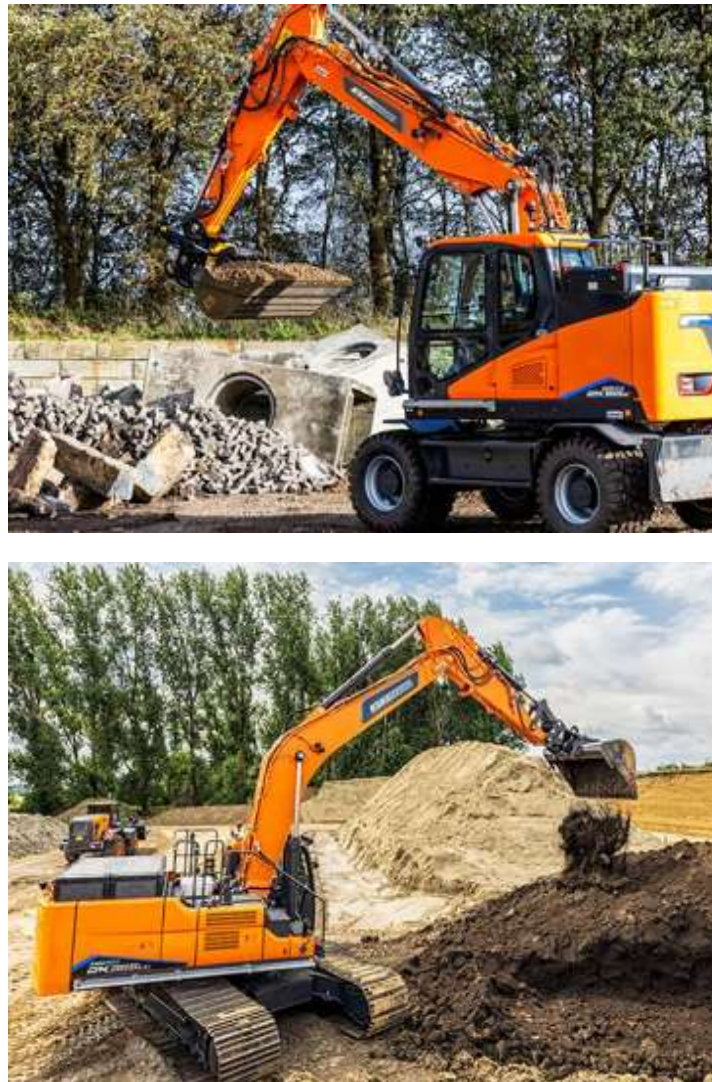
Figure 1.1 –DX165W (top) and DX355LC (bottom). These two electric excavators were used in the TNO study to collect energy consumption data for heavy-duty zero-emission construction. The DX165W (17-ton wheeled) represents a medium-sized vehicle based on SEB categories, while the DX355LC (35-ton tracked) is classified as large. Source: TNO (2024), “Technische eindrapportage Bouwplaats van Morgen”, P11947.
