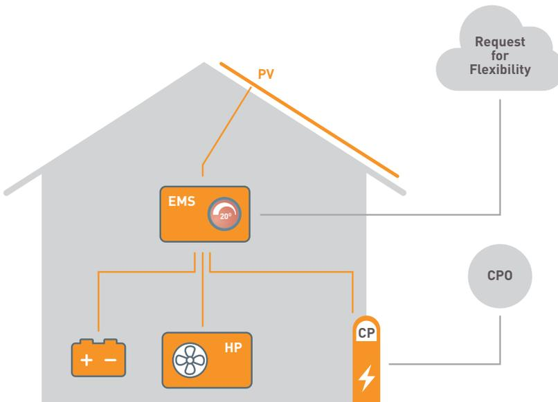
Combining different devices is a good strategy to deliver the requested flexibility. The dominant idea for unlocking flexibility from in-home devices is that devices are not controlled individually, but that an Energy Management System (EMS) in the home ensures connectivity with the devices. An EMS “interconnects” the devices and provides flexibility access to the requesting parties.
