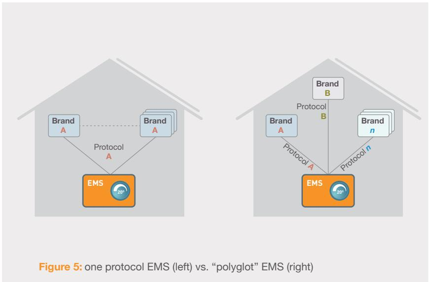
**Figure 5:** one protocol EMS (left) vs. “polyglot” EMS (right)
