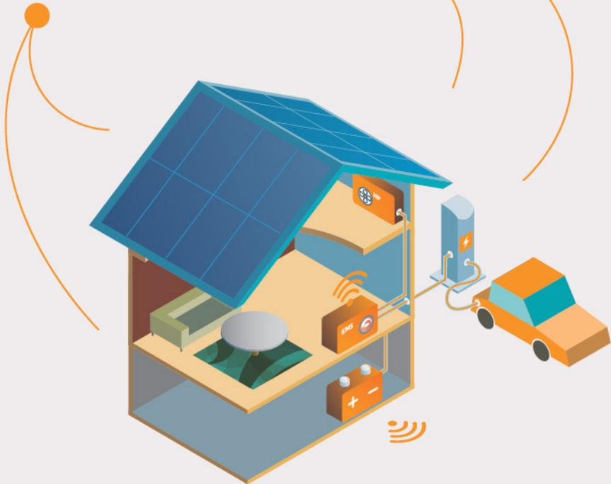
A dense installation of solar panels in a neighborhood cause peaks in local electricity generation, electric cars cause a simultaneous and substantial power demand. And other devices, such as heat pumps and inductive cooking, can also cause a simultaneous peak demand. However, many of these devices also offer control possibilities; unlocking flexibility from these devices.
