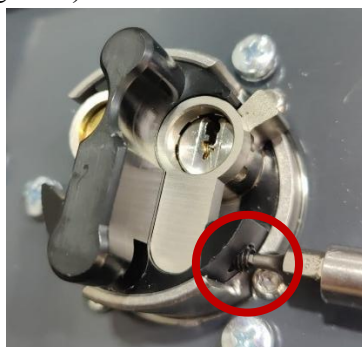
Figure 5 - Locking cylinders from the old access door which should be transferred to the new DUO Wide access door.
