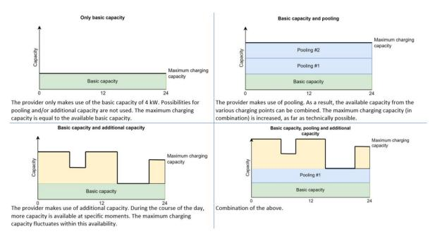
1) Basic capacity per charging point: As the first building block, users and providers can assume a guaranteed basic capacity of 4 kW per charging point, for the charging of an EV.
