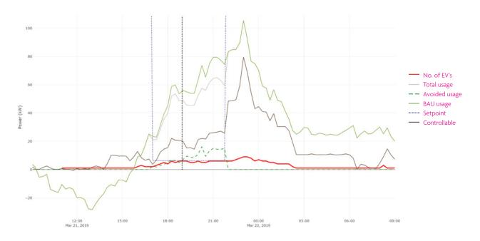
Figure 12: Visualization of load profiles for static charge management
