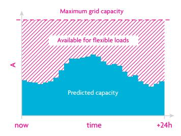
Figure 7: Maximum grid capacity vs. predicted capacity and flexible loads
