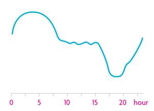
Figure 3: Example daily dynamic control signal for EV charging
