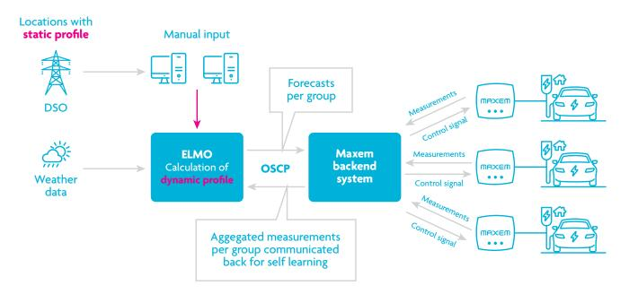
Figure 6: Overall technical architecture
