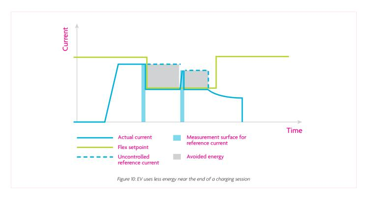
Since the avoided energy cannot be *measured*, the method described above was developed to *calculate* it. Because the firmware was adapted to handle these three scenarios, researchers can make an accurate calculation about the actual impact of charge management.
