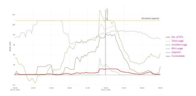
Figure 11: Visualization of load profiles for dynamic charge management
