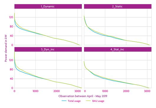
Figure 22: Duration curves of total usage and BAU usage with maximum constraint
