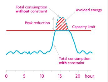
Figure 5: Determining how charge management reduces peak load
