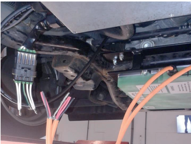
Figure 9: Connecting output of secondary coil with input of rectifier (left) and output of rectifier with input of onboard charger (right). Orange DC fast charging cables disconnected and tape wrapped
