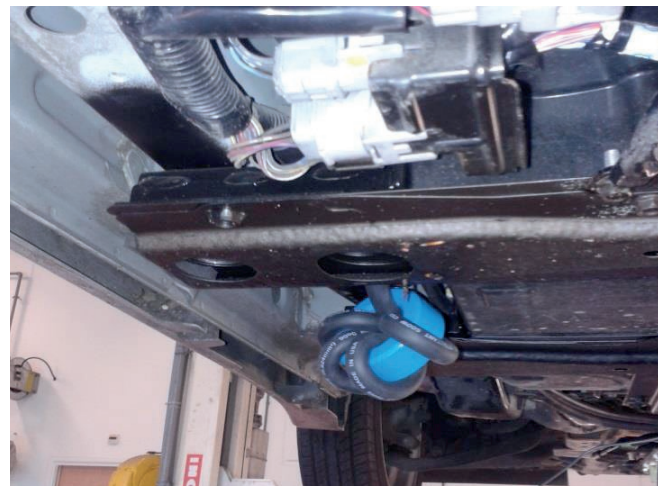
Figure 10: Plugging new communication line of rectifier into the existing one in the onboard charger (left). Wrapping communication line around a ferrite core (right)
