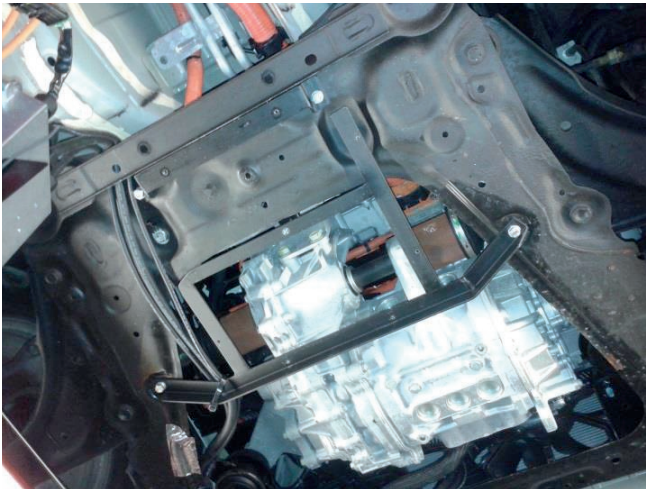
Figure 7: Mounting bracket and position of secondary coil under the vehicle
